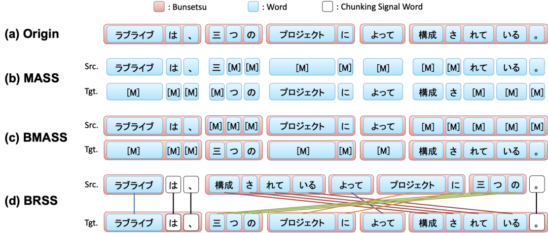
Figure 4: An example of source and target for MASS, BMASS, BRSS with the meaning “LoveLive is made of three projects.”
